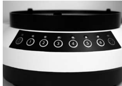
FIG. 6. There are eight buttons on the selection panel on the front of the instrument. Buttons 1-6 correspond to cartridge positions on the cartridge holder. A LED light indicates the chosen reagent strips.
