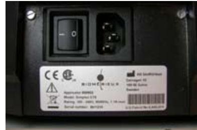
FIG. 5. The main switch on the back of the instrument is used to turn the power supply ON or OFF. The power cord socket and the identification label are placed on the back of the instrument.
